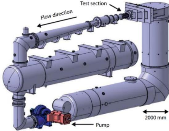
Figure 1 Cavitation tunnel
