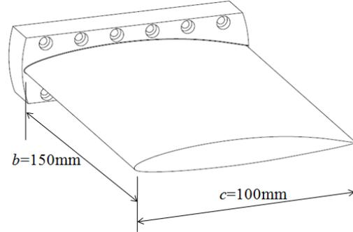
Figure 2 NACA66 hydrofoil
