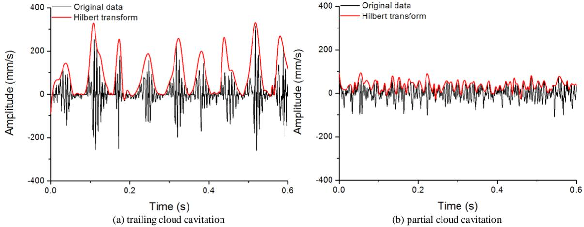
Figure 6 Time evolution of the vibration velocities
