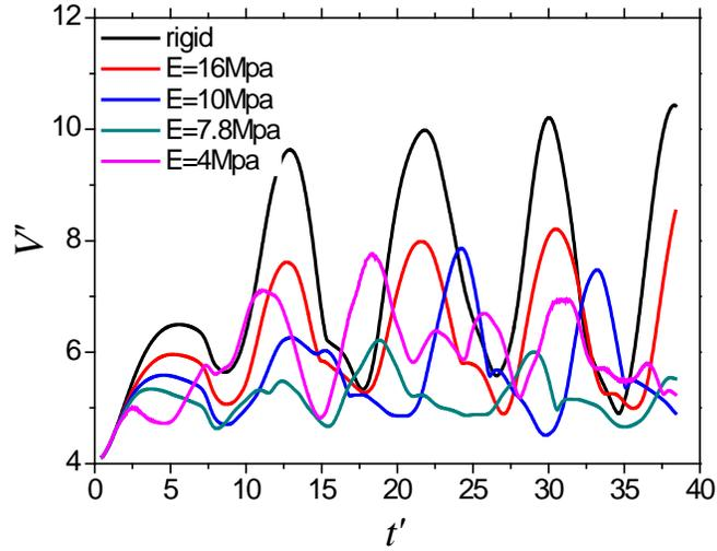
Figure 5: Comparisons of cavitation volume with different Young's modulus.
