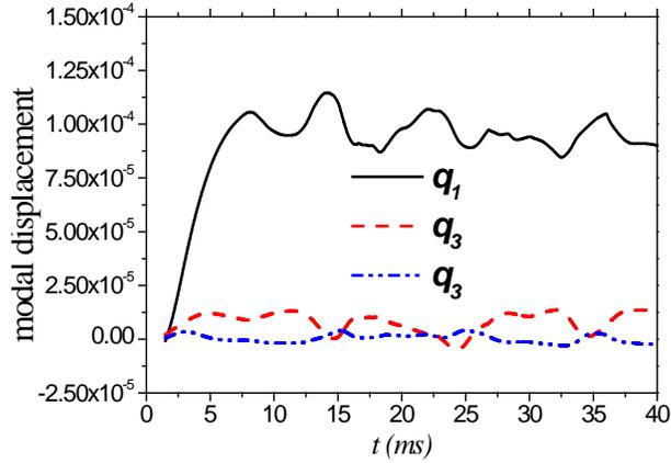
Figure 3: Modal displacement with  $E = 10$  Mpa
