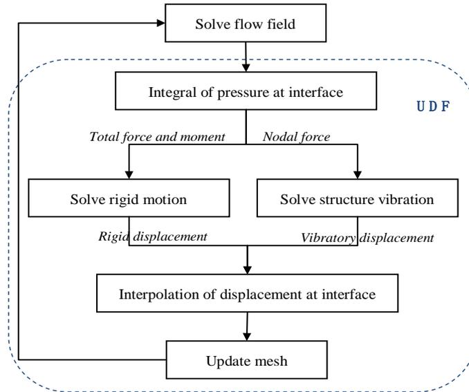
Figure 2: Block diagram of fluid-structure coupling method
