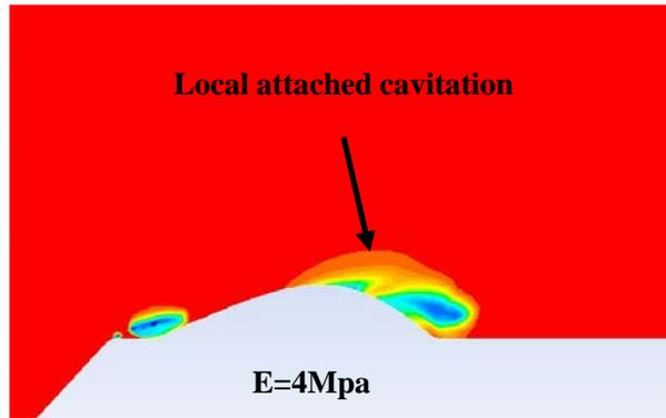
Figure 6: Growth of local attached cavitation ( $E = 4$  Mpa).
