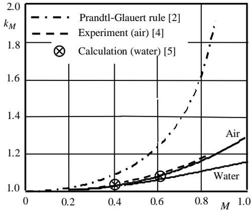
Fig. 1 Effect of the Mach number on hydrodynamic load of a profile
