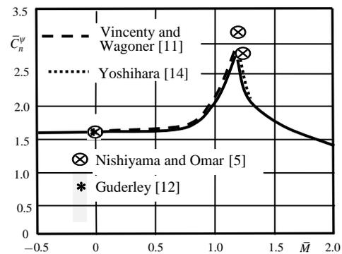
Fig. 4 Hydrodynamic load on the profile at transonic gliding with the running pitch angles below  $2.6^\circ$
