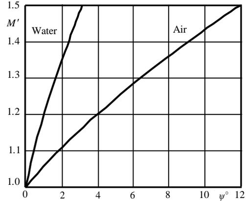
Fig. 2 Effect of a running pitch angle  $\psi$  on the Mach number  $M'$  of the shock wave attachment
