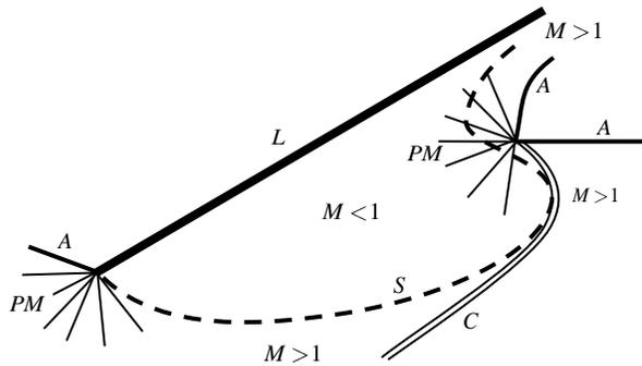
Fig. 3 The planing profile with the detached shock wave
