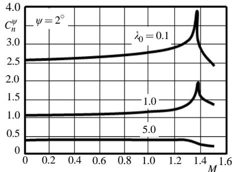
Fig. 5 Hydrodynamic load on plates at gliding with the attaching of the shock wave
