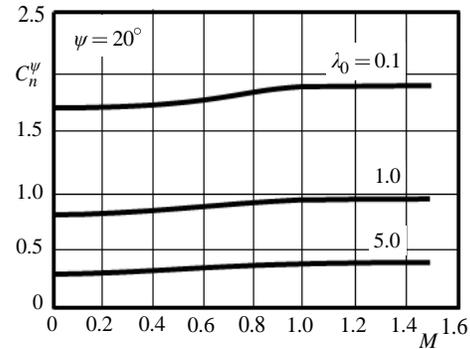
Fig. 6 Hydrodynamic load on plates at gliding with the detached shock wave
