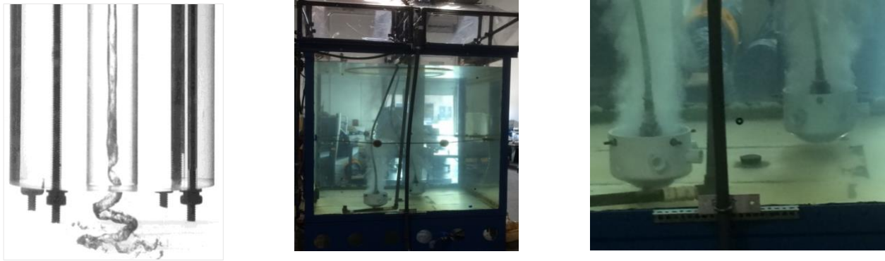
Figure 1. Cavitation Core from DYNASWIRL ® nozzle (left hand photo). Large (1,350 gallon) test tank with 2 bubble generators (center hand photo). Close-up of the generators at the bottom of the tank (right hand photo).
