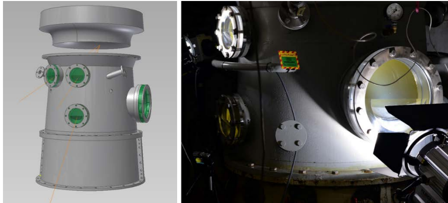
Figure 2. (a) Outline of the acrylic-glass windows mounted on the draft tube with the adequate vision angle to see the blades; (b) photograph showing the flow visualization tests.
