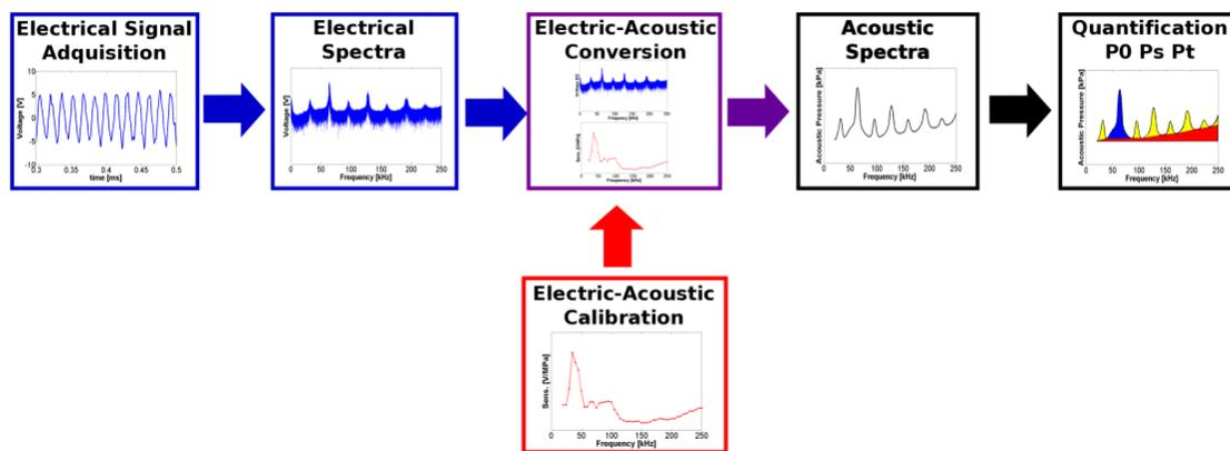
Figure 2. Processing steps to quantify the cavitation acoustic parameters.
