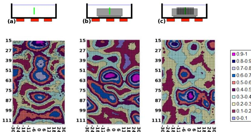
Figure 5. Loading effects on acoustic uniformity 40 kHz batch system (a) empty tank, (b) added an empty cassette and (c) added 14 disks to the cassette.
