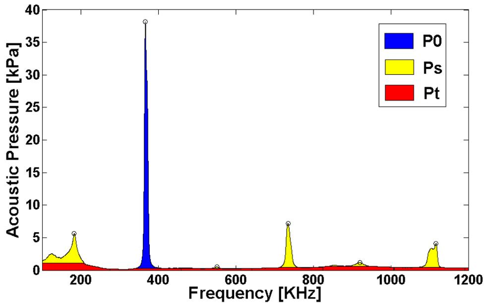
Figure 1. Acoustic pressure spectrum example. The blue area represents the direct field pressure ( $P_0$ ) generated by the driving source at its fundamental frequency ( $F_0$ ). The yellow areas represent harmonics, sub-harmonic and ultra-harmonics associated with stable acoustic cavitation pressure ( $P_s$ ). The red area represents the broadband noise generated from the collapse of bubbles, or transient cavitation pressure ( $P_t$ ).
