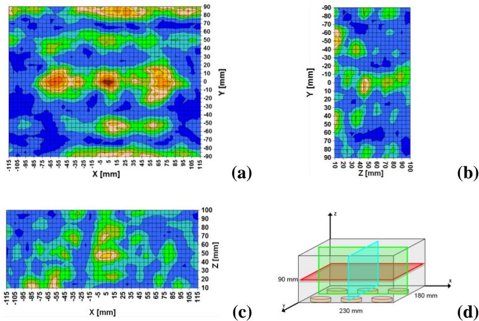
Figure 4. (a) Normalized  $P_0$  uniformity mapping for XY plane, (b) YZ plane and (c) XZ plane and (d) Schematic of cleaning tank showing scanned planes.
