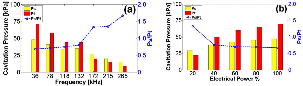
Figure 3. (a) Stable and transient cavitation comparison at different frequency. (b) Stable and transient cavitation readings in a 78 KHz tank as a function of the electric power.
